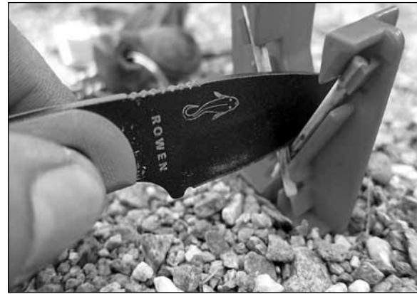
When it comes to sharpening, a simple ceramic crock stick sharpener is all that is needed to keep the edge of the Candiru factory sharp.
